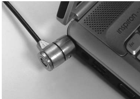
FIGURE 5.12 A cable in the security slot keeps the laptop from leaving easily.
